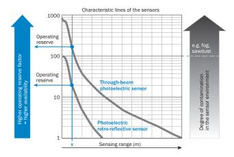
At a sensing range of "x" the photoelectric retro-reflective and through-beam photoelectric sensors have different operating reserves (see blue arrow). The higher the operating reserve factor, the better the sensor can compensate the contamination in the air or in the light beam and on the optical surfaces (front screen, reflector), i.e. the sensor has the maximum availablity, otherwise the sensor switches due to pollution although there is no object in the path of the light beam.
