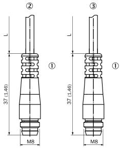
For length of cable (L), see technical data ① Cable with connector M8
