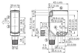
$\textcircled{\sc 0}$  Standard direction of the material being detected
