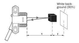
ZTB18-xxxxxx**D02**: x = 47 mm / y = 4 mm ZTB18-xxxxxx**D04**: x = 93 mm / y = 8 mm ZTB18-xxxxxx**D06**: x = 139 mm / y = 12 mm
