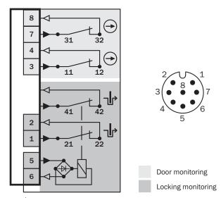
$\ensuremath{ \mbox{\fontfamily Positive}}$  Positive action N/C locking monitoring contact
