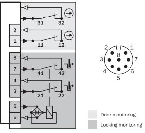
$\neg\!\!\!\!\!\mathrm{Jr}$  Positive action N/C locking monitoring contact  $\boxdot$  Positive action N/C door monitoring contact
