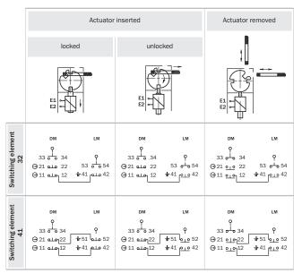
${}_{\ensuremath{\mathbf{W}}}$  Positive action N/C locking monitoring contact
