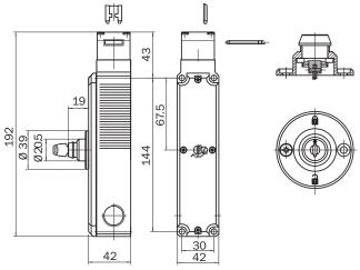
The mechanical unlocking mechanism of the i10 Lock can easily be operated via a key. The lock on the front of the i10 Lock is fixed with two screws.
