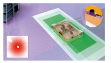
Wide field of view of 276° (270° + 6°) The wide field of view of the picoScan100 allows a large working range. With two diagonally aligned sensors, it is even possible to cover 360° – and do so with little mounting and alignment effort.
