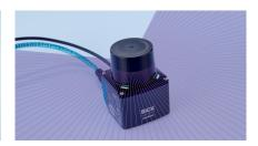
Improved detection options The large working range (75 m at 90% remission) and the high angular resolution (up to 0.05°) of the picoScan100 enables small objects or fine structures to be detected even at large distances. This makes the sensor suitable for accurate localization or reliable collision avoidance.
