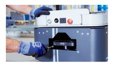
SICK also considered simple installation when designing scanGrid2. The sensor is mounted to the vehicle with only two screws.
