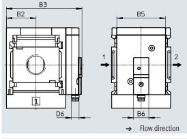
[AD11], [AD12] Pressure sensor with LCD display
